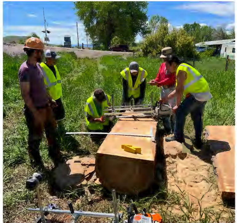
Training in use of portable Alaska Sawmill in Wyola (June 9, 2022). Credit: Jamie Kirby
